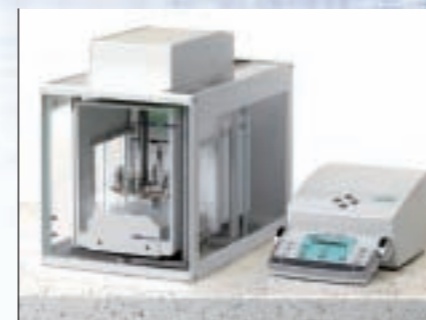
AX107H The automated nano comparator up to 100g.
