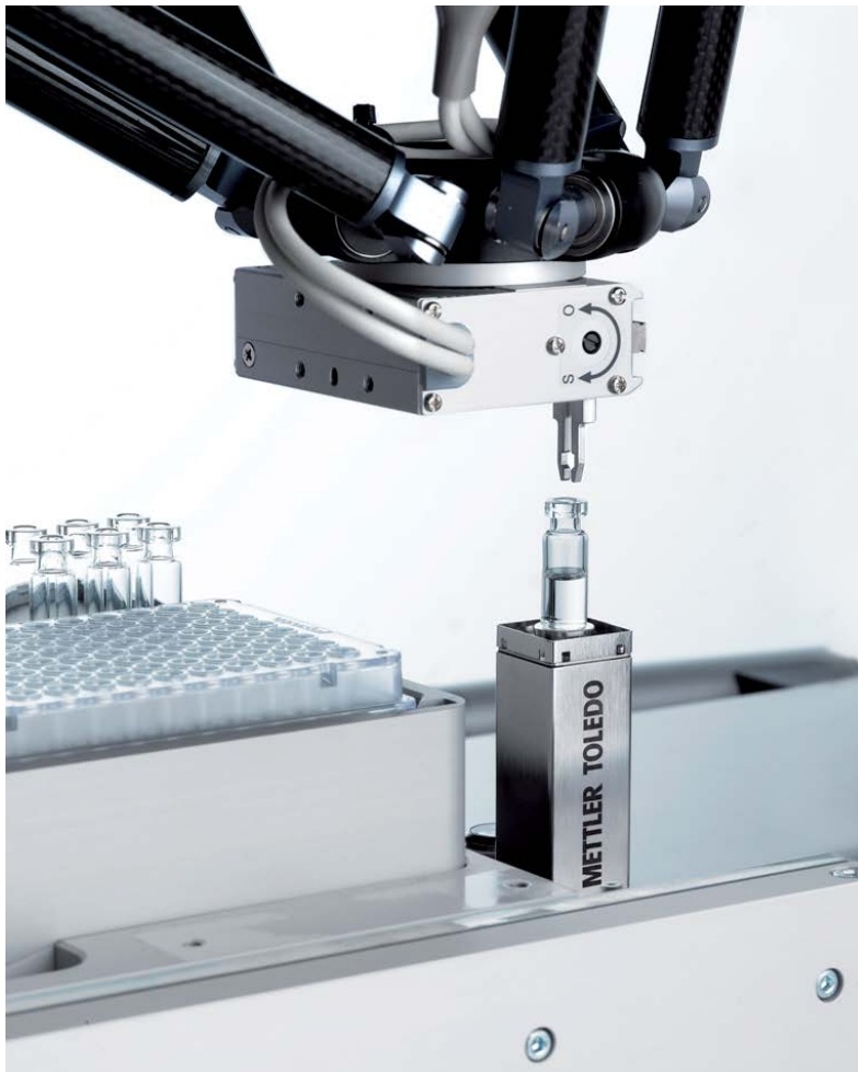
Figure 3-5: Good practice for applying & removing weighing objects Weighed object is placed on the weighing pan gently with a robotic arm. This way, vibrations and shocks can be minimized and the stability can be reached within shortest time
