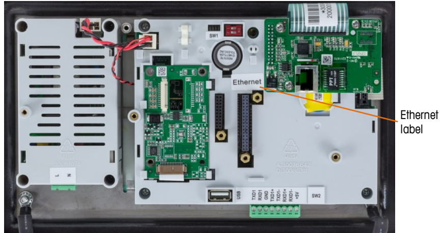
Figure 2-36: Ethernet Option Installed on Main Board
