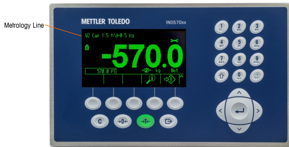
Figure 2-63: Metrology Line on IND570 Display
