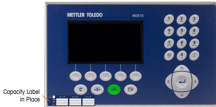
Figure 2-65: Capacity Label Installed
