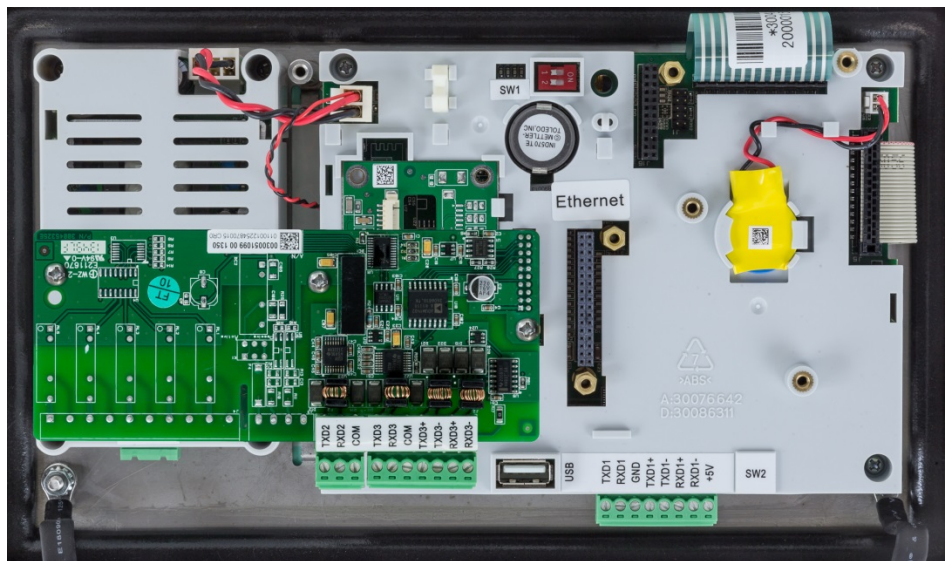
Figure 2-39: COM2/3 Option Board, Installed
