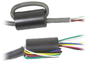
Figure 2-18: Installing the Ferrite Cores
