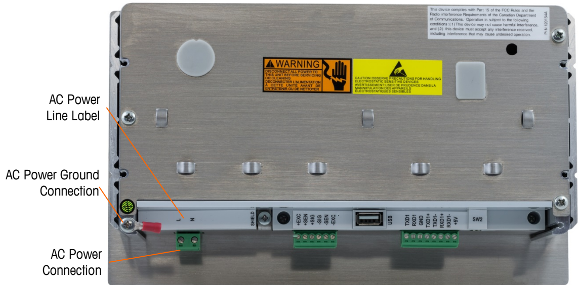
Figure 2-26: AC Power Connection on Panel Mount
