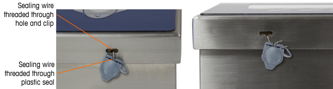
Figure 2-70: Harsh Enclosure Seal Threaded and Ready to be Closed – Standard Orientation (left) and with Panel Reversed (right)
