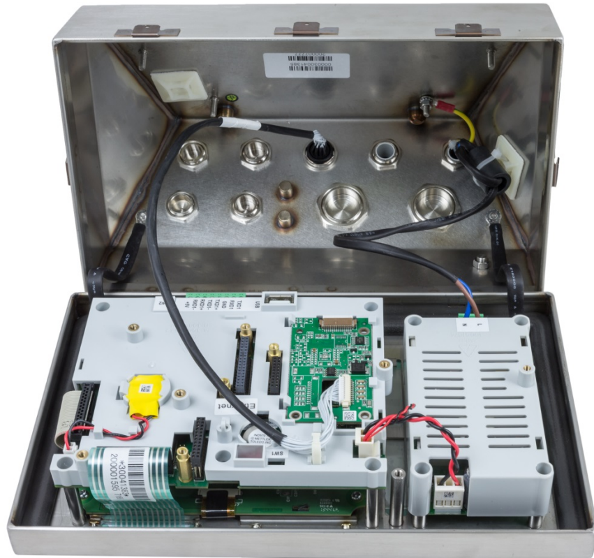
Figure 2-15: Front Panel and Load Cell Connection Reversed
