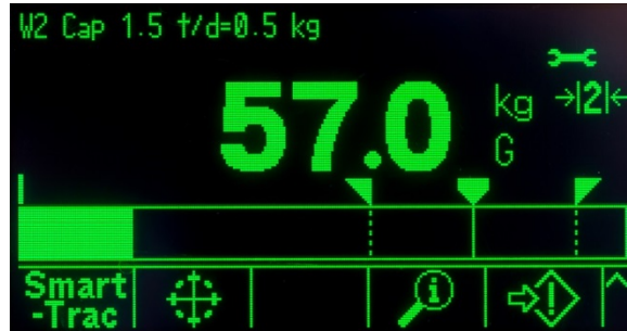
Figure 1-11: Small Material Transfer SmartTrac Enabled
