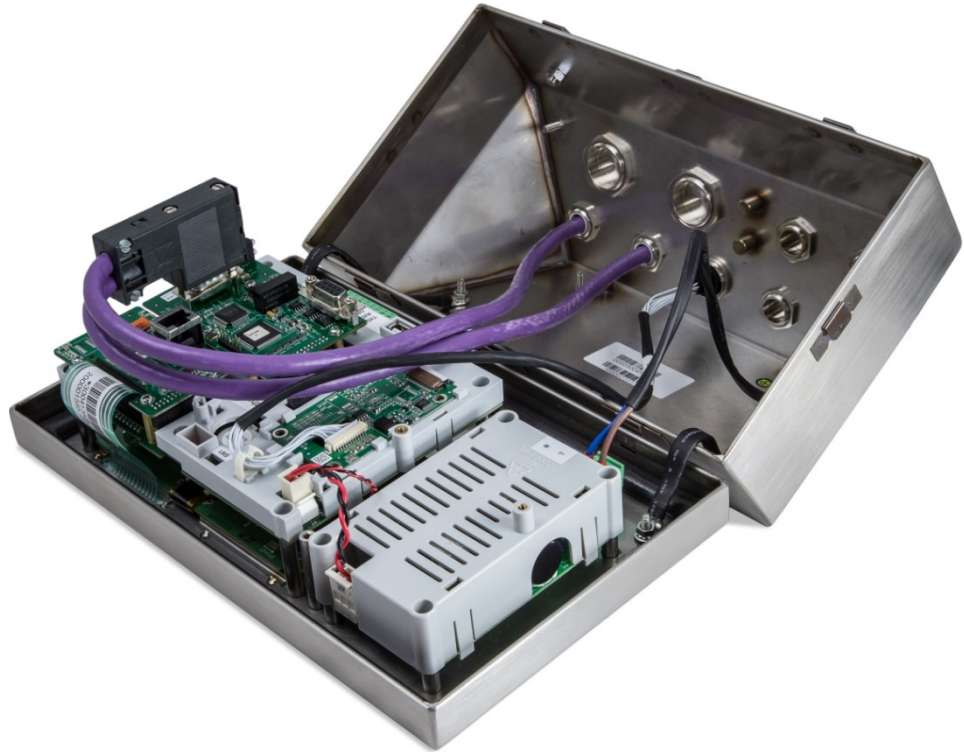
Figure 2-56: PROFIBUS Cable Connection in Harsh Enclosure
