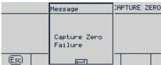
Figure 3-13: Zero Calibration (Failed)
