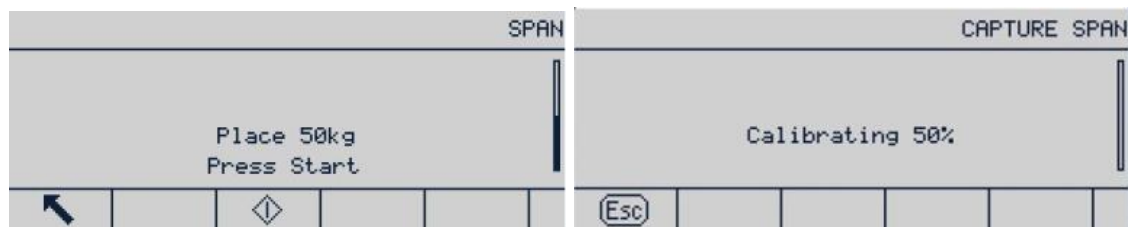
Figure 3-15: Span Calibration in Progress
