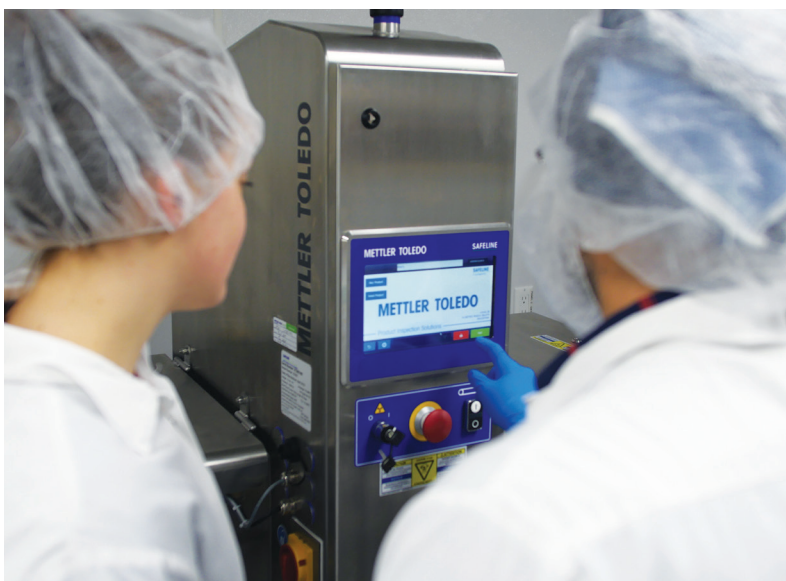
All finished gelato and sorbetto products are run through the Safeline X33 X-ray Inspection system to check for any possible contaminant.
