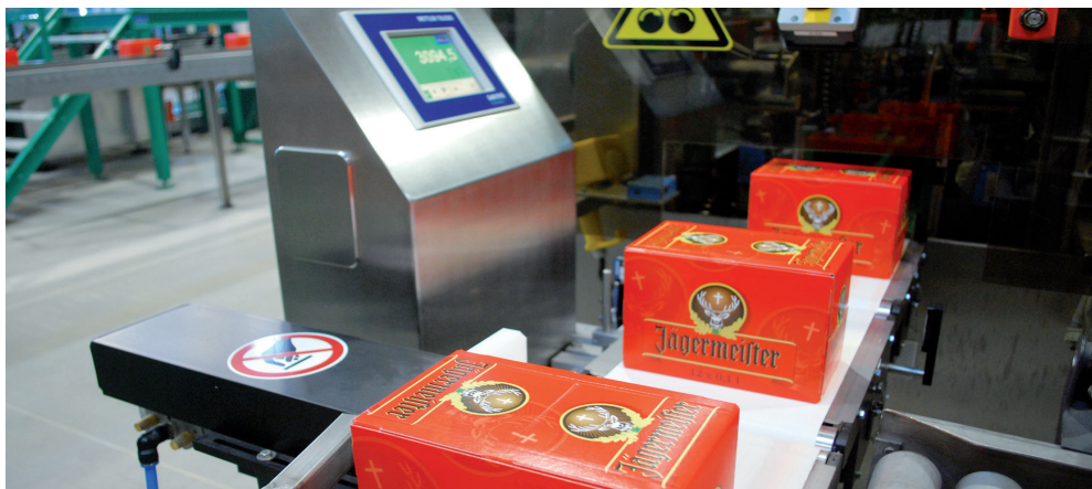
METTLER TOLEDO in-line checkweigher examining completeness of cartons with bottles
