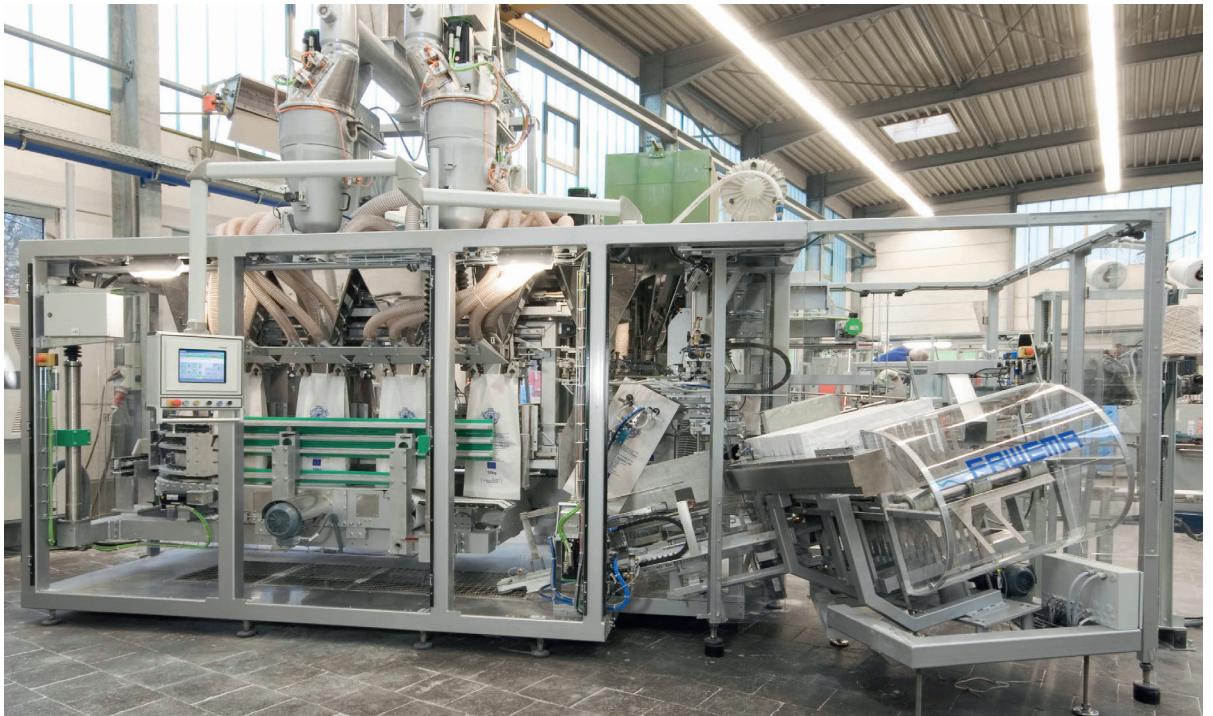
Fawema has integrated the checkweigher (see photo below) into a line featuring a packaging machine for single and meslin flour, where it checks the filling and packaging process
