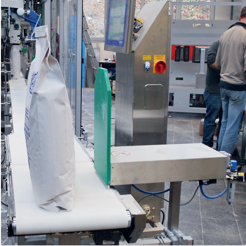
Sacks of flour that do not conform to tolerance limits are reliably rejected by a pusher
