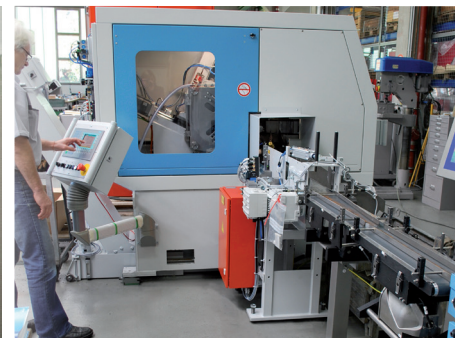
The Siemens SIMATIC control is the interface between the checkweigher and the Behringer-Eisele HCS90 sawing system
