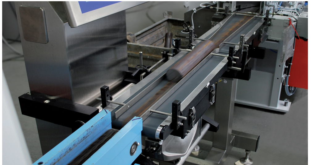
With high accuracy, the checkweigher reliably controls an upstream steel sawing system
