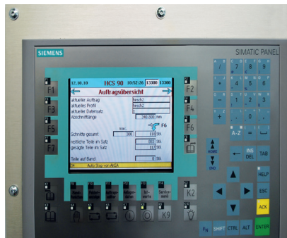
The Siemens SIMATIC control is the interface between the checkweigher and the Behringer-Eisele HCS90 sawing system
