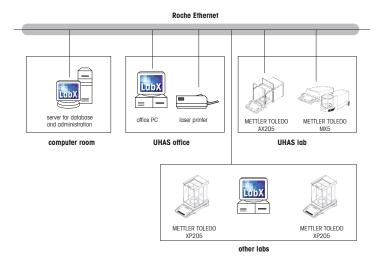
The flexible software architecture allows installation on multiple computers in different rooms. LabX controls multiple balances directly over the network.
