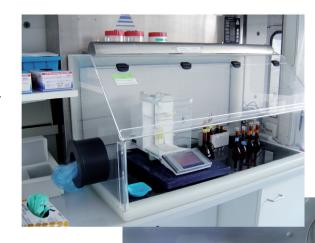
The METTLER TOLEDO balances operate under stringent conditions in ventilated cabinets.
