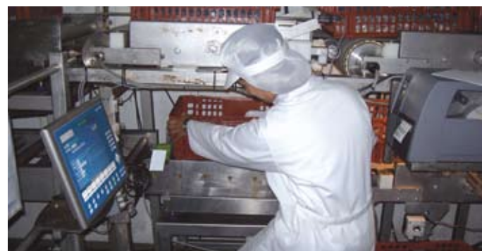
Box weighing installation with IP69k protected weighing terminal and PBA430 weighing platform
