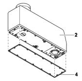
2 Attach long base plate to weigh module (2) using 4 M5 screws.
