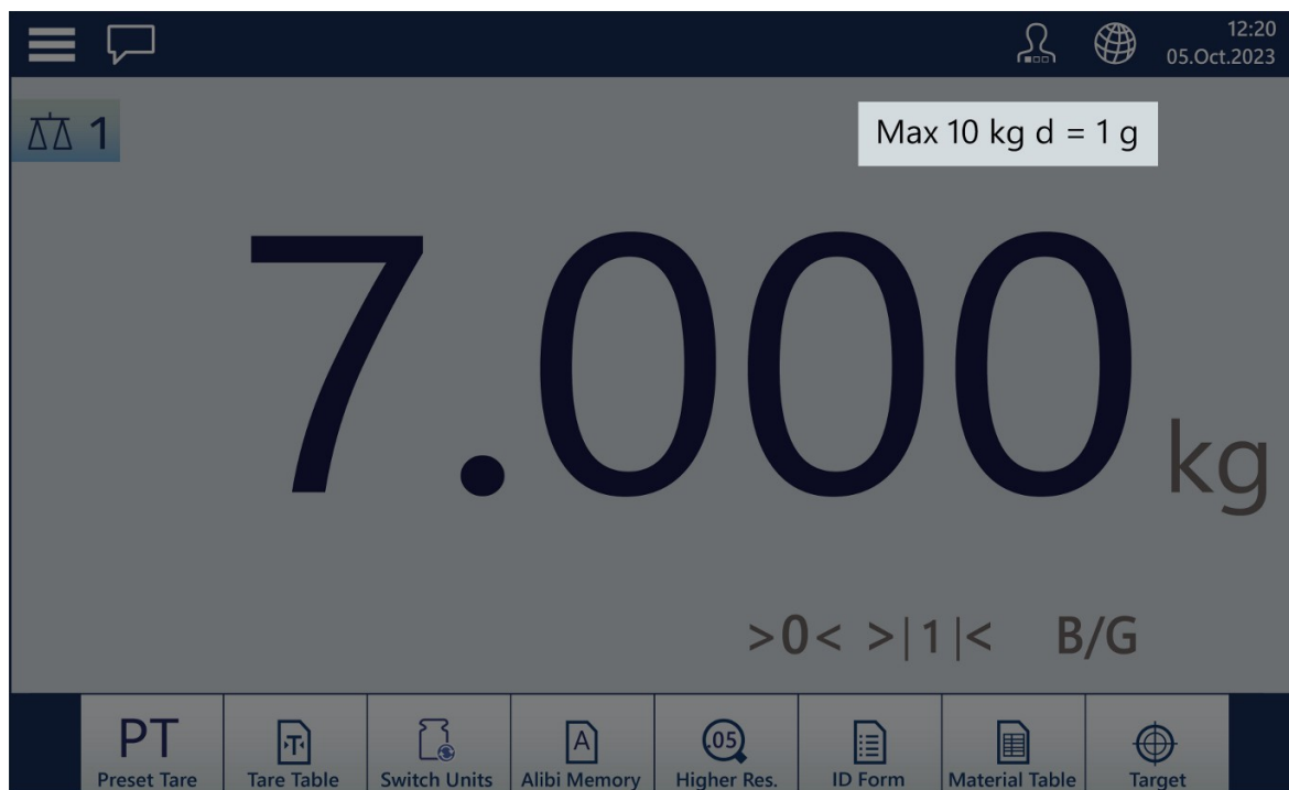
Figure 46: Metrology Display Area
