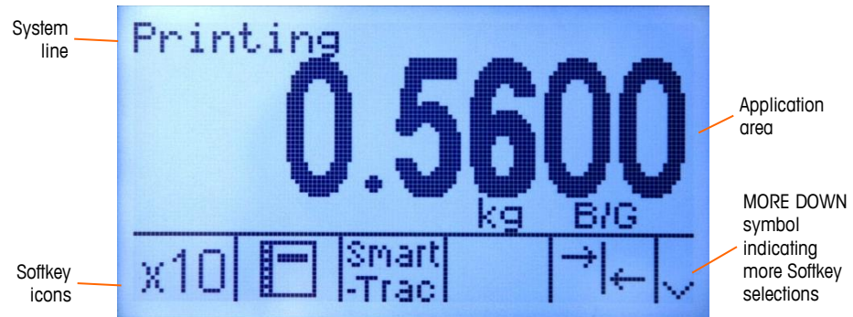
Figure 2-9: Default Home Screen, System Line with Message Showing
