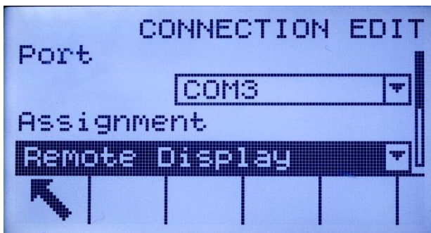
Figure 3-10: COM2/COM3 Connection Configured for Remote Operation
