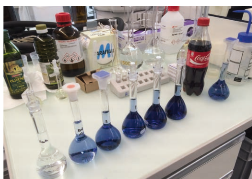
Figure 31: Series of prepared phosphate standard solutions
