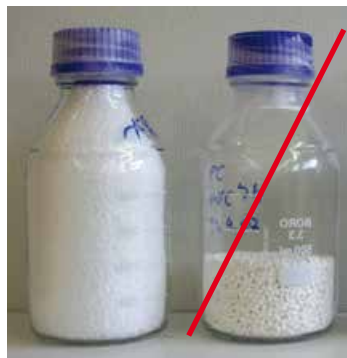
Fig. 4: Filling of sample containers. Left: Ideal filling. Right: Fill level too low.
