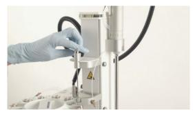
3 Connect the fitting nut to the needle and screw the fitting nut in until you hear a "click".
