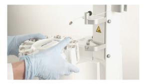
3 Align the blue arrow on the rack with the blue arrow on EasySampler 1210.
