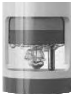
Sensor cleaning with air using the cavitation effect.
